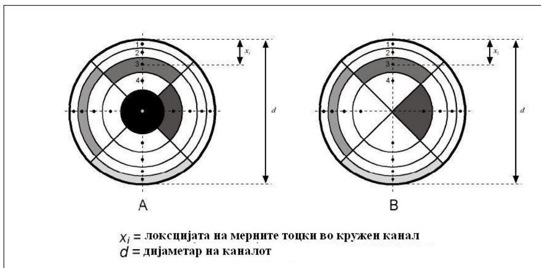
Figure 4. The locations of the measurement points in a circular duct , methods A and B (SFS-EN 13284-1, source Finnish Handbook for Emission Measurements)
